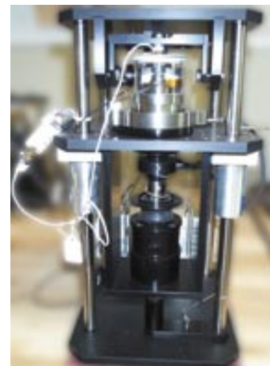
Figure 3 Front view of a custom Cervical Spine Simulator
